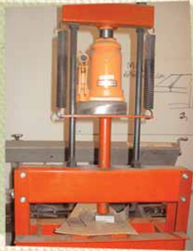
Place aluminum on press with stamp facing down on top of it. Center both under rod.
