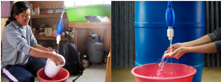
Figure 3. Balde a Balde portable faucet, by Kim Chow, provides running water from any bucket, to maximize cleanliness while optimizing water use, for people living without basic services. Prototype testing in Cerro Verde, Lima, Peru.
