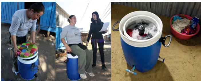
Figure 2. Techo staff field testing refined GiraDora clothes-washer/spin-dryer prototype by Alex Cabunoc and Ji A You, in campamento near Santiago, Chile.
