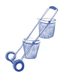
Inexpensive, lightweight, and easy-to-roll water dolly for the common 5 gallon bucket
